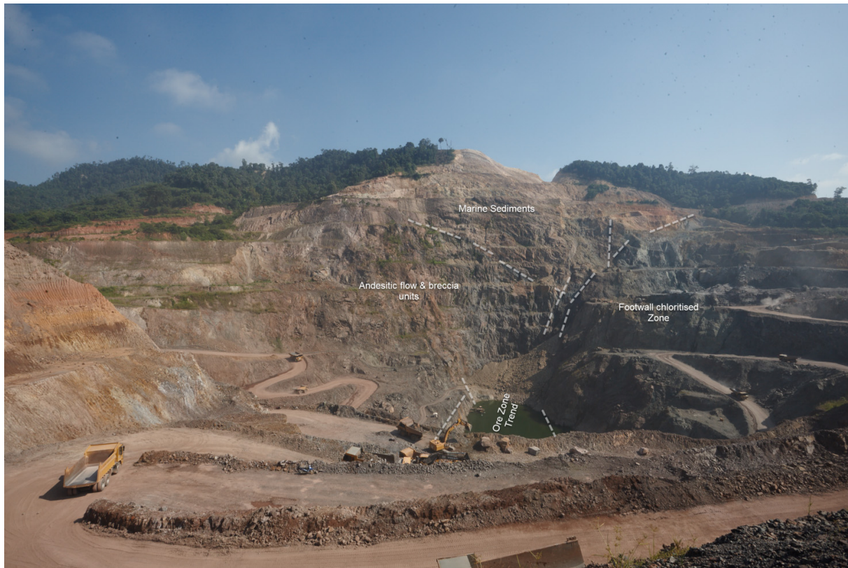
Figure 6, View looking NW, capping marine sediments over hosting andesitic volcanics
