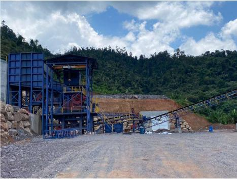
Figure 9: View of our 600 tonne per hour primary crushing plant
