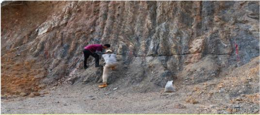
Figure 8: Composite Channel Sampling Across Quartz Veins
