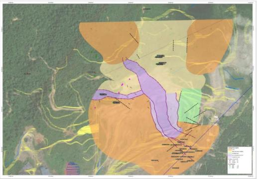
**Figure 2,** Key local scale geological & structural features of the Chaah deposit. Note, the discovery of Andesite porphyry directly west of the deposit, this unit is magnetite bearing and hosts late-stage quartz-sulphide veining. The porphyry ranges from fresh to variably hydrothermally altered
